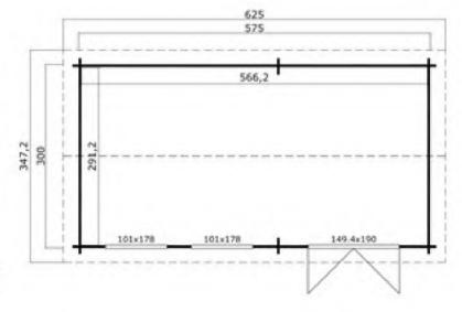
Roof Slope 15° Treated Bearers 70 x 45mm
